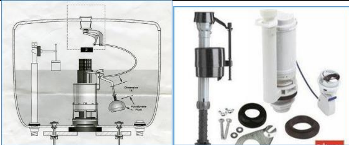
Dual flush cistern system
