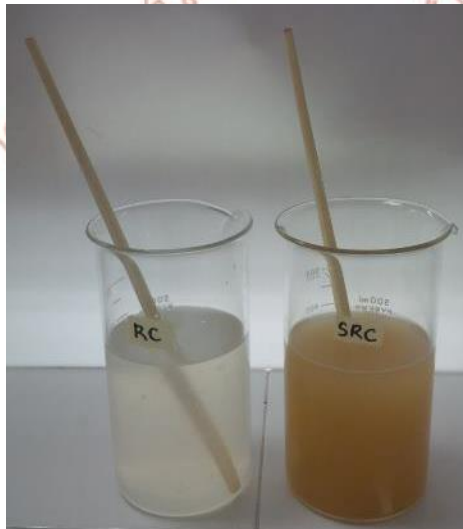
Picture 2. Refined Carrageenan and Semi-Refined Carrageenan Diluted in fresh water, RC is clearer than SRC
