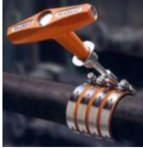
Steel coupling connectors being tightened using a torque wrench
