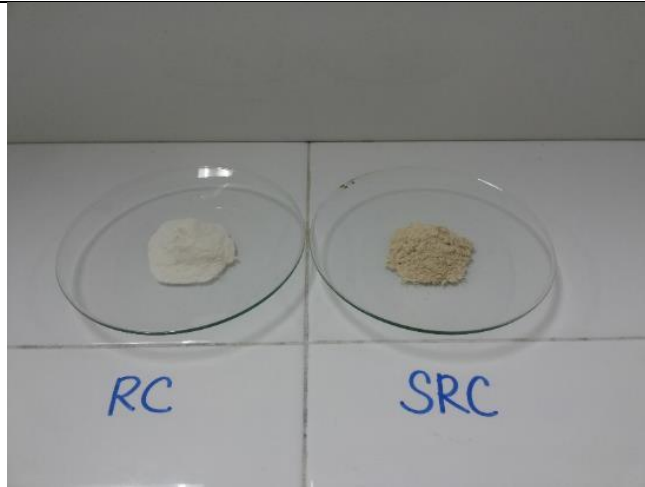
Picture 1. Refined Carrageenan (RC) and Semi-Refined Carrageenan (SRC) Powder In powder form, RC is whiter than SRC
