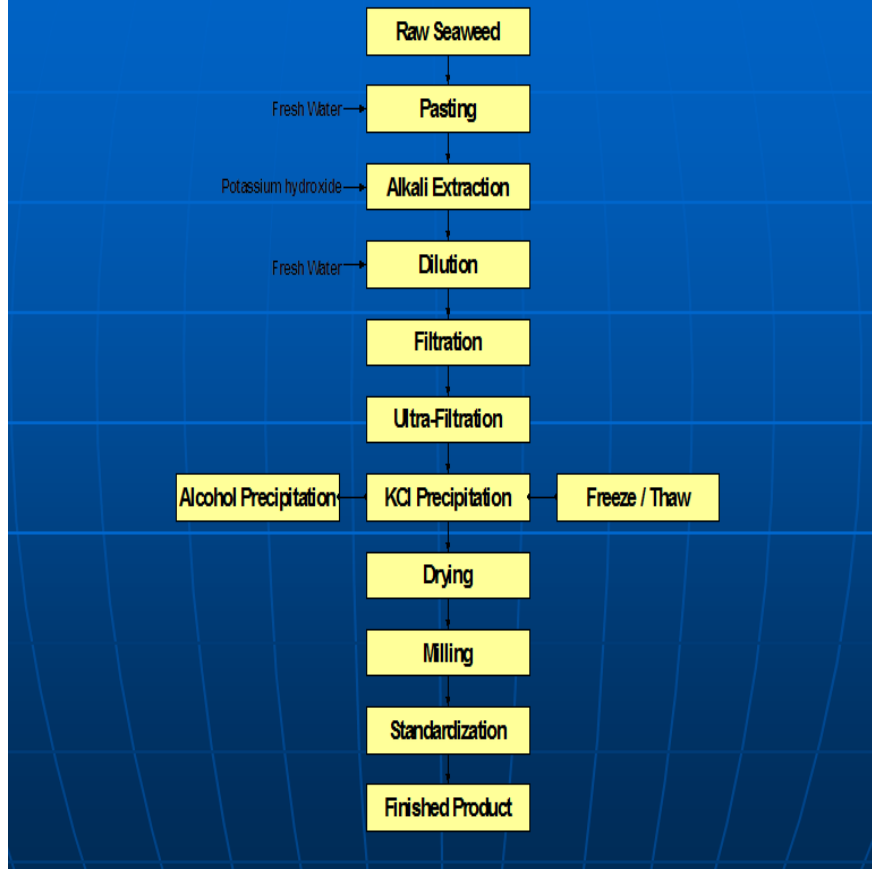
Picture 4. Manufacturing Process of Refined Carrageenan (Source: Indonesia)
