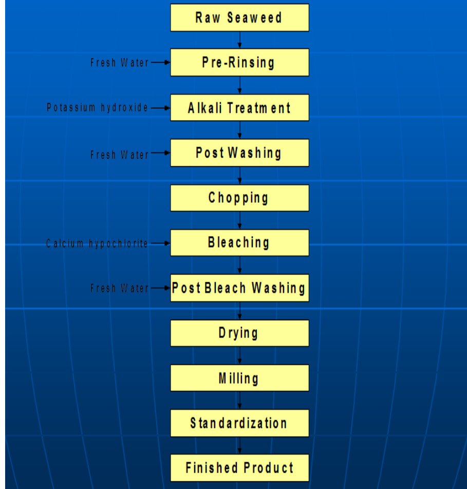
Picture 3. Manufacturing Process of Semi-Refined Carrageenan
